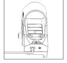
side of your sight. To move your point of impact to the left, with the provided hex key, turn the adjustment counter-clockwise. Each click is equal to 1 MOA. To move the point of impact to the right turn the adjustment clockwise.
