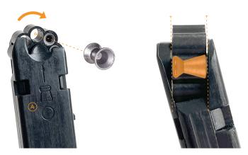
Insert pellets or steel BBs into the chamber of the rotary clip located at each end of the magazine and then rotate the clip clockwise until all chambers are loaded. When loading pellets, ensure the pellet is inserted nose first from the back of the magazine indicated by the ammunition marking (A). The pellet must be fully seated into the chamber so that it is flush with the rear of the rotary clip and does not extend past the front.
