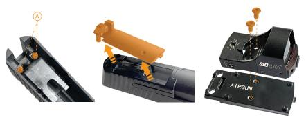
The SIG Air Reflex Sight (sold separately) will come with the appropriate Airgun optics plate required to mount the reflex sight to the P229 air pistol.
