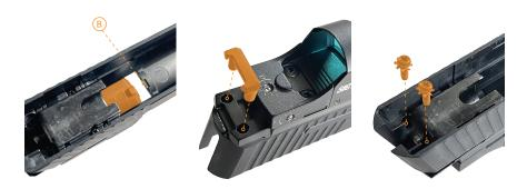
Place the SIG Air Reflex Sight and Airgun Optics Plate assembly onto the slide and ensure that the plate seats into the notch (B) under the front of the sight plate opening. Replace the rear sight with the included optics plate anchor to allow proper clearance to access the reflex sight locking screws.
