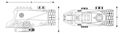
A -6.3 in / 159mm B - 2.6 in / 67mm C - 3.2 in / 82mm
