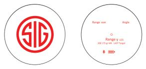
The startup screen with the SIG logo can be exited at any time by pressing the RANGE or MODE buttons. The startup screen can also be permanently deactivated using the MENU system on your KILO or using the BDX App in the RANGEFINDER > SETTINGS page.
