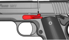
5. Push the slide stop lever out of the frame from right to left.
