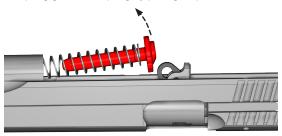
8. Rotate the barrel bushing counterclockwise and remove it from the slide. Rotate the barrel link forward.
