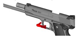
9. Align disassembly notch on slide and push slide stop remaining way into frame.
