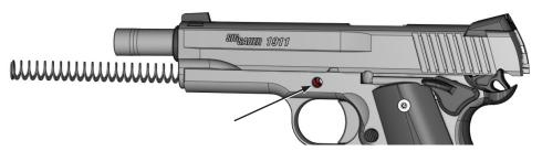
8. Insert slide stop shaft through frame so it passes through barrel link.
