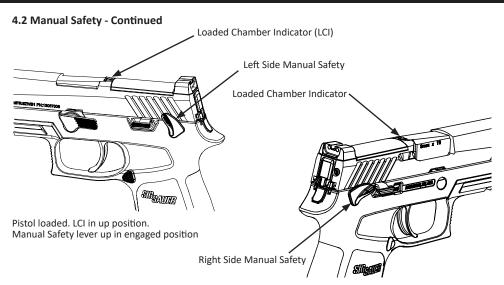
Pistol unloaded. LCI down. Manual Safety lever in down disengaged position.
