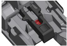
MAGAZINE DISCONNECT MECHANISM SPRING INSTALLED
