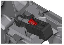
MAGAZINE DISCONNECT MECHANISM SPRING DISLODGED
