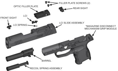
\*The magazine disconnect mechanism grip module is compatible with any FCU equipped with a manual safety. Magazine disconnect mechanisms are only available in California compliant FCU's. 126
