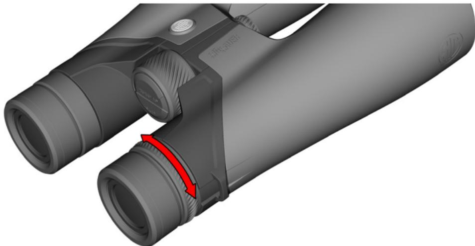
Your binocular is now focused for your eyesight. To make any adjustments in the field, simply turn the center focus dial while viewing through both barrels.
