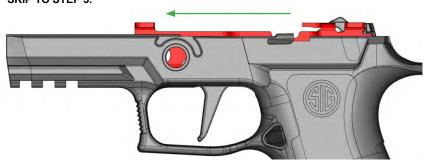
4. To overcome the magazine disconnect for disassembly, access the magazine disconnect mechanism through the magazine well of the grip module. Slightly lift the magazine disconnect while applying pulling on the trigger, allowing it to clear the rectangular cutout in the grip module.
