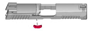
Insert the extractor pin, extractor spring, and extractor plus pin into the channel on the right side of the slide. Ensure the flat surface of the extractor pin rests on the post of the extractor.
