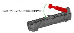
b. For X5 Legion, insert guide rod into spring then compress spring while inserting the guide rod and spring into slide. Head of spring guide should rest against barrel lug.
