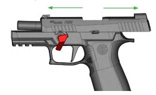
Guide the complete slide assembly (slide, barrel, recoil spring, and guide) forward and off of the frame.
