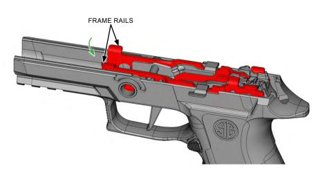
Insert the takedown lever (turn and push simultaneously) through the grip module and FCU, locking the fire control unit in place.
