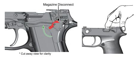
5. Pull up on the frame rails, then rotate the FCU up and out from the grip module.
