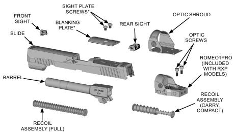
\* Blanking plate and screws included with XSERIES RXP. Optional on standard RXP models.
