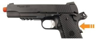
In addition to the thumb safety, the 1911 is also equipped with a grip safety. The grip safety is automatically engaged when there is no pressure being held against it. When the pistol is held firmly by the grip, the grip safety is depressed which disengages the safety allowing the trigger to be pulled.
