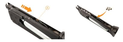
Pull the magazine's follower (A) to the bottom of the track and lock it by tilting it outwards so that it braces against the track's lip. Load the BB's into the round opening in the track just above the follower. Continue to load the BB's until approximately half a BB's width extends into the round opening. Then, push the follower inwards and slowly let it travel up until it contacts the last BB.
