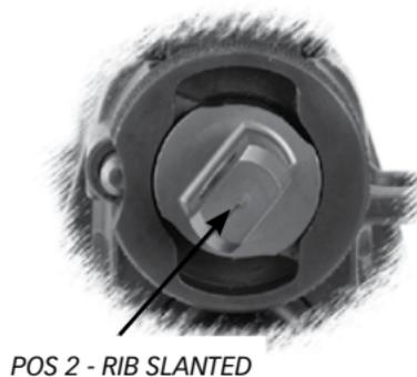
When cycling or ejection problems are encountered due to heavy fouling, the gas valve can be moved to Position 2 by rotating clockwise as far as the stop. In this position, a larger gas volume is released against the operating rod. The need to use the gas valve in Position 2 is an indication that the rifle requires cleaning.
