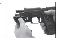
The Adapter Clamp Assembly should be seated as close to the front of the trigger guard as possible while still maintaining a positive lock with the rail stop. Make sure the holes in the Polymer Adapter Clamp line up with the rail slots on the pistol. Insert the "L" shaped Adapter Rail Lock to guarantee placement. Adapter Rail Lock should only be inserted from the right side.
