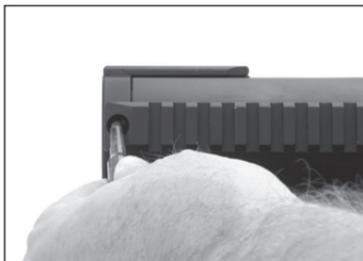
Slide the Front Polymer Adapter Clamp onto the accessory rail of the pistol.
