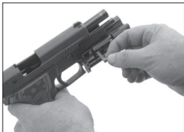
Hold the ACP by the top rail and insert the pistol and Adapter Clamp Assembly into the corresponding rails located inside the front of the ACP.
