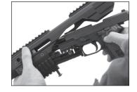
Push the pistol as far forward as possible and slide the Adapter Clamp Assembly retaining pin back into the adapter.
