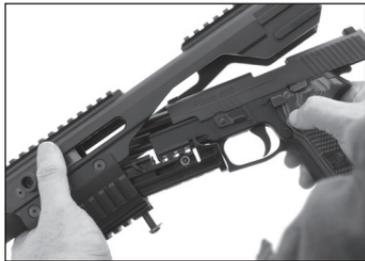
Replace the Rear Locking Assembly by sliding it back onto the rear of the ACP. Insure you have the correct Rear Polymer Adapter Clamp installed for your pistol, as shown in the photo.
