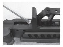
2.5 Install the front (long) Chassis screw hand tight with 5mm hex.
