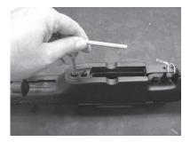
1.2 Remove the rear stock screw using the 5mm hex wrench and separate action from stock.
