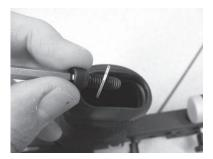
3.2 Tighten the grip screw using the 3/16 Hex Wrench.
