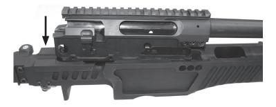
2.3 Coat both new Chassis screws, supplied with the chassis, with a small amount of Loctite #243.
