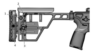
1 -Quick Detach Sling Cup 2 -Comb Clamp Lever
