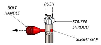
5. Release pressure on the striker shroud and pull the handle out to release the striker from the bolt carrier.
