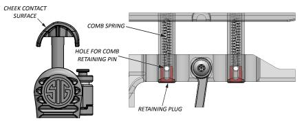
STOCK FRAME AND COMB ASSEMBLY SHOWN TRANSPARENT FOR CLARITY
