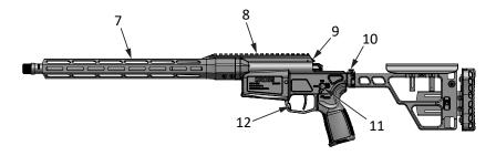
7-Handguard 15 Inch 8 -MIL-STD 1913 Rail 9 -Bolt Catch 10 - Stock Lock Button 11-Ambidextrous Safety Selector 12-Magazine Release
