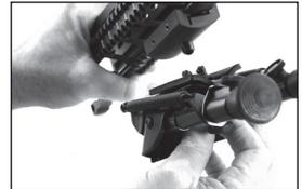
13. Tighten by rotating the knurled locking wheel on the bi-pod clockwise until snug.
