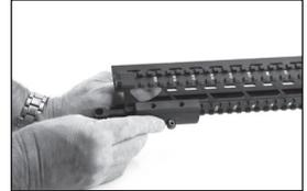
8. Slide the two mounting screws through the adapter and start to thread them into the adapter. Tighten the two (2) mounting screws until snug while pushing the adapter forward on the rail. Failure to push the adapter forward while tightening will result in the adapter moving from recoil as the rifle is fired.
