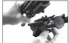
5. Tighten by rotating the knurled locking wheel on the bi-pod clockwise until snug.
