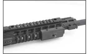
3. Slide the two mounting screws through the adapter and start to thread them into the adapter. Tighten the two (2) mounting screws until snug while pushing the adapter forward on the rail. Failure to push the adapter forward while tightening will result in the adapter moving from recoil as the rifle is fired.
