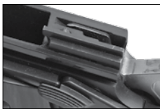
Fig 4: Plunger lever in the down position ready for assembly.
