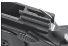
Figure 5: Plunger lever in the up position.
