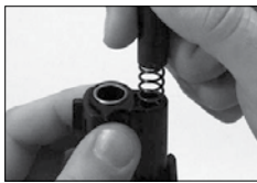
Fig 2: Releasing the recoil spring
