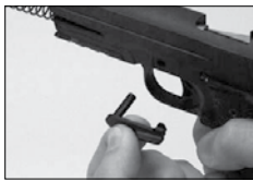
Fig 3: Removing slide stop
