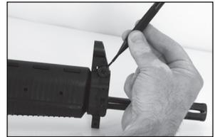
Use punch for alignment of hole and pin.
